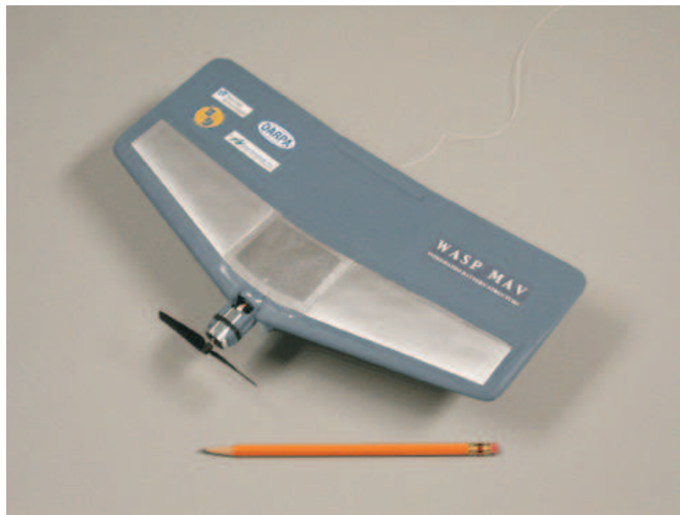
Figure 3.8 The WASP Micro Air Vehicle (35)
