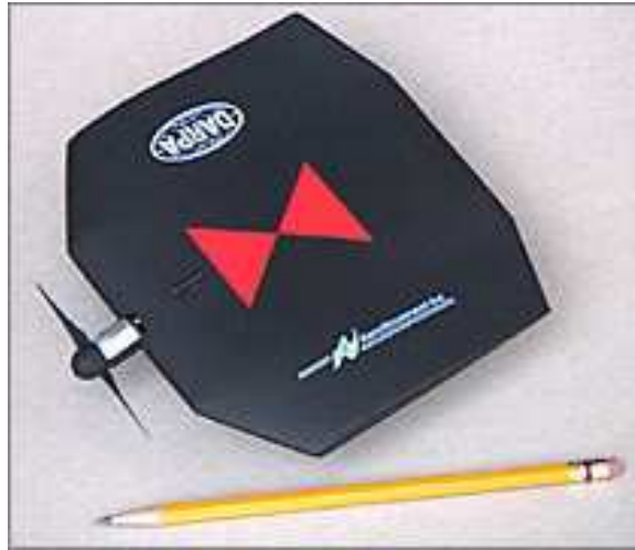
Figure 3.7 The Black Widow Micro Air Vehicle (2)
