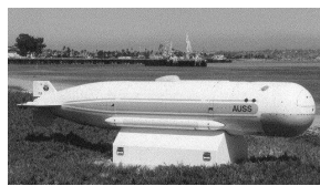
Figure 3.2 Advanced Unmanned Search System (42)
